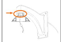
Use the Allen key and a hex head cap screw to assemble and firmly affix the camera's pendant cap to the bracket.
