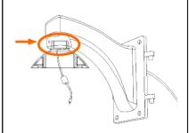
Follow camera instructions to assemble the pendant cap. Use the Allen key and a hex head cap screw to assemble and firmly affix the camera's pendant cap to the bracket.
