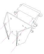
When using a power box, screw power box onto the pole adapter.
