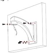
Affix the bracket to the wall using the appropriate screws and screw anchors (not provided).
