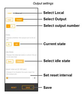
If an optional washer pump is connected to pins 3 and 4 (Alarm-Out A1 and A2) on the camera's 14-pin terminal block connector, the washer controls on the <u>Wiper Page</u> activate it through local output 1. For information about how to configure local output 1 to activate the washer pump, see <u>Install and Test the Optional Wash Kit</u>.
