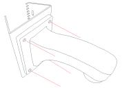
When using a wall mount bracket, affix the wall mount bracket onto the pole adapter.
