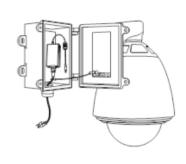
Buckle up the safety rope, make the camera connections, tighten the two hex screws to seal the box, and then complete assembly.
