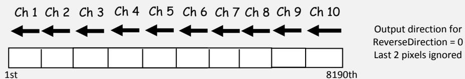
The CameraLink standard requires a minimum of 256 Pixels per channel. Then for the versatile model and the lowest definitions, some combination sensor Mode / Output mode are not available. The following table details the possible combinations :
