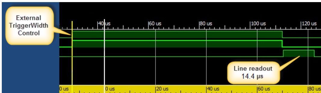
Figure 47: External Trigger Width Exposure
