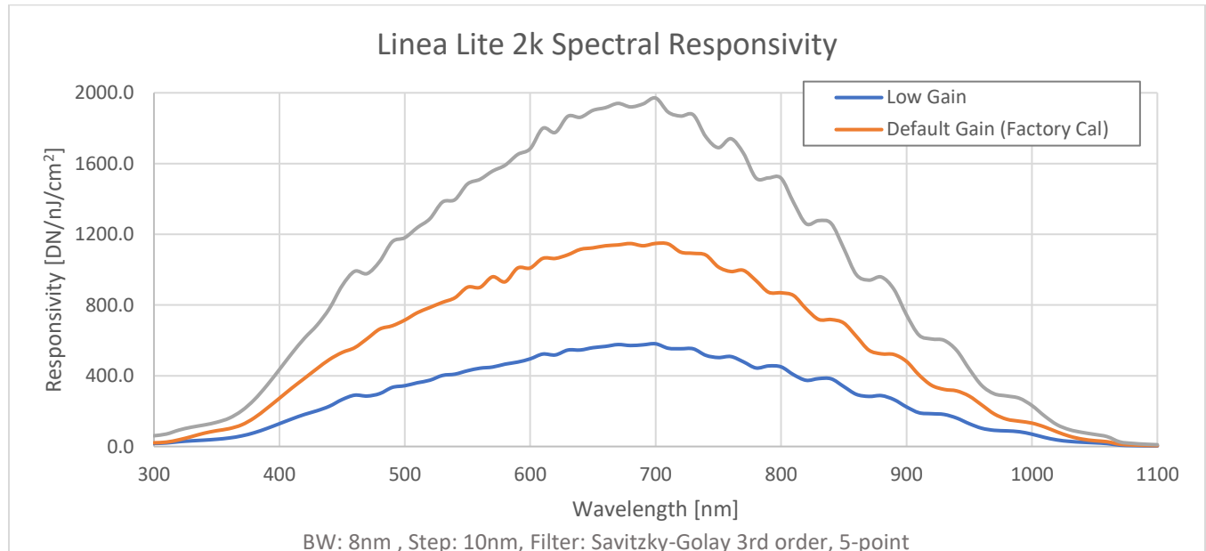
Figure 2: Linea Lite 2k Spectral Responsivity
