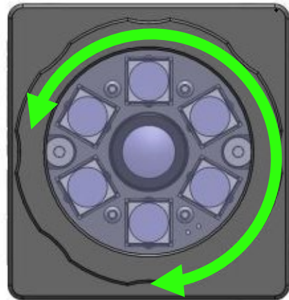
M12 cover rotates to adjust focus
